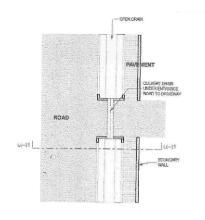
The diagram shown on the left shows what we currently have in Nairobi. The open drains allow easy access for rubbish to enter leading to a blocked drain. When the drains are blocked, water cannot pass through. This stagnant water attracts mosquitoes. In order to allow the water to constantly flow, we need to cover the drains to reduce rubbish inside the drains. In this case we assume that the road is cambered and sloped, to allow a constant flow of water.
